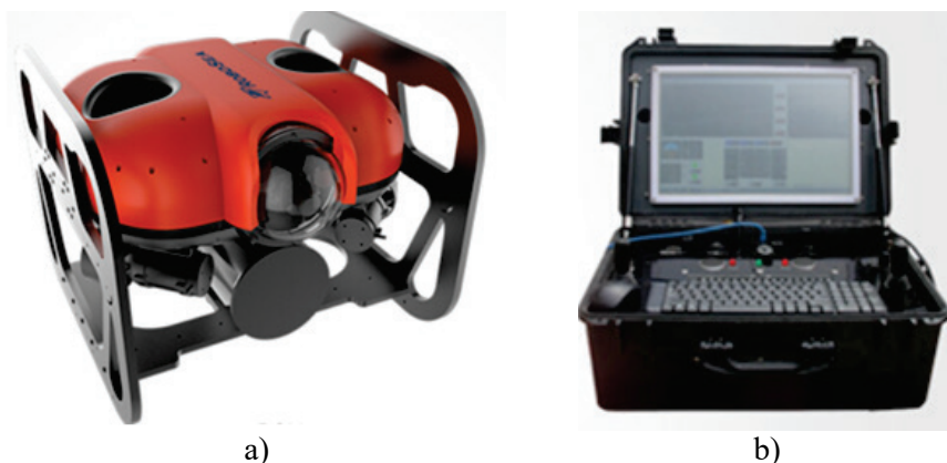
Figure 3 – Underwater system with self-propelled submarine "ROBO-ROV": a) – ROV; b) – Control panel
